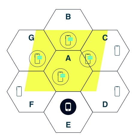
The yellow shading (the polygon) is the target area defined by the alert originator. It includes cell sites A, B, C, D, F and G. But the polygon doesn't include cell site E. Based on the target area, the identified cell sites will broadcast the alert for this geometric shape. All mobile devices in those target sites will receive the alert.
